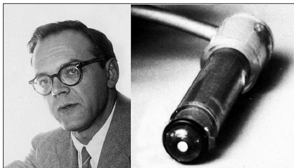
Fig. 2. Leland C. Clark, Ph.D. (1918–2005), a steroid biochemist at Fels Research Institute, Antioch College, Yellow, Springs Ohio. His polarographic membrane covered oxygen electrode (right) was manufactured by the Yellow Springs Inst. Co., and disclosed publicly by Clark on April 18, 1956 at a meeting of interested physiologists at the annual meeting of biologists in Atlantic City, N. J.
